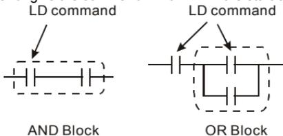
The structures of command LDP and LDF are similar to the command LD. The difference is that command LDP and LDF will act in the rising-edge or falling-edge when contact is ON as shown in the following.
