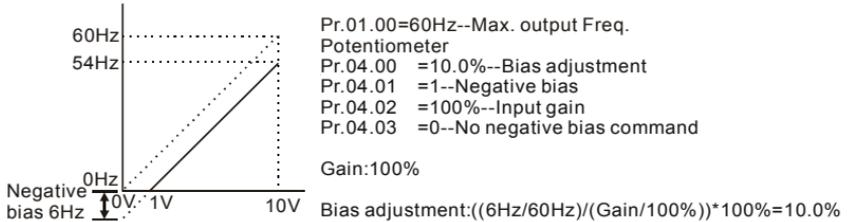
**Example 6: Use of negative bias in noisy environment and gain adjustment to use full potentiometer range**
