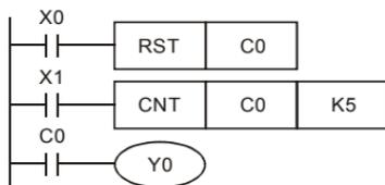
1. When X0=On, RST command is executed, C0 reset to 0 and output contact reset to Off.
