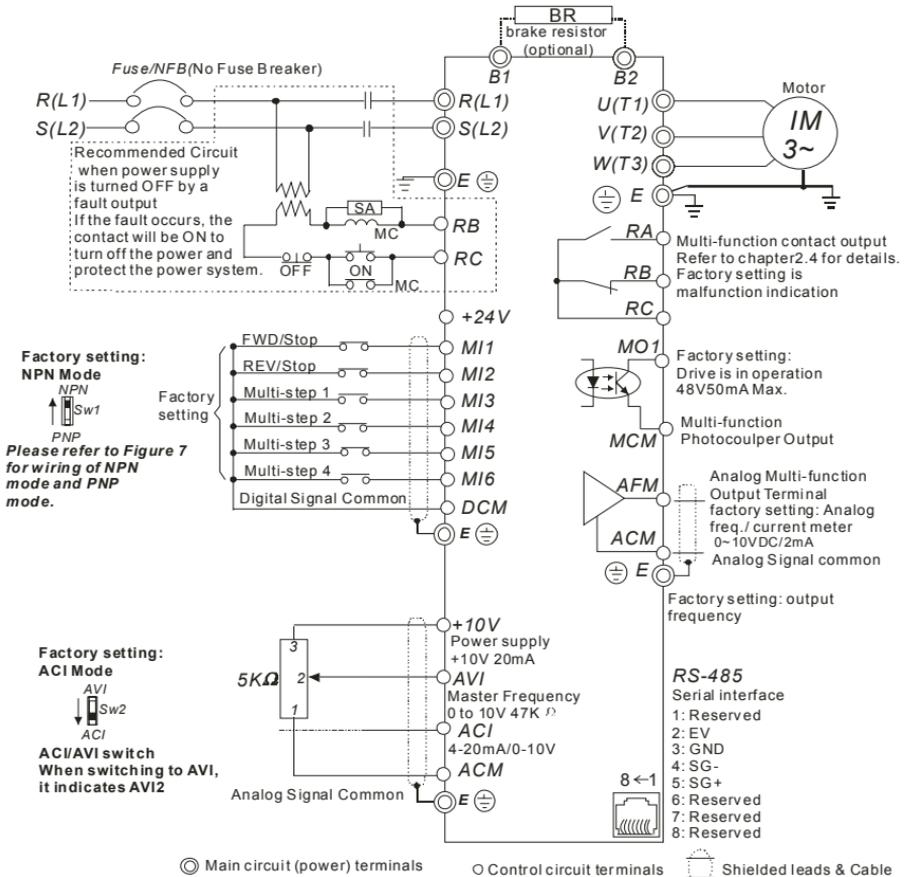
**NOTE** For VFD-E-T series, the braking resistor can be used by connecting terminals (B1 and B2) directly. But it can't connect DC-BUS in parallel.
