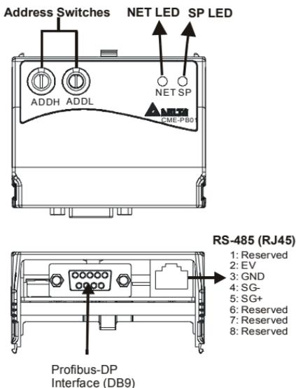
1. SP LED: Indicating the connection status between VFD-E and CME-PD01.
