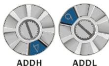
CME-PD01 has two rotary switches for the user to select the PROFIBUS address. The set value via 2 address switches, ADDH and ADDL, is in HEX format. ADDH sets the upper 4 bits, and ADDL sets the lower 4 bits of the PROFIBUS address.
