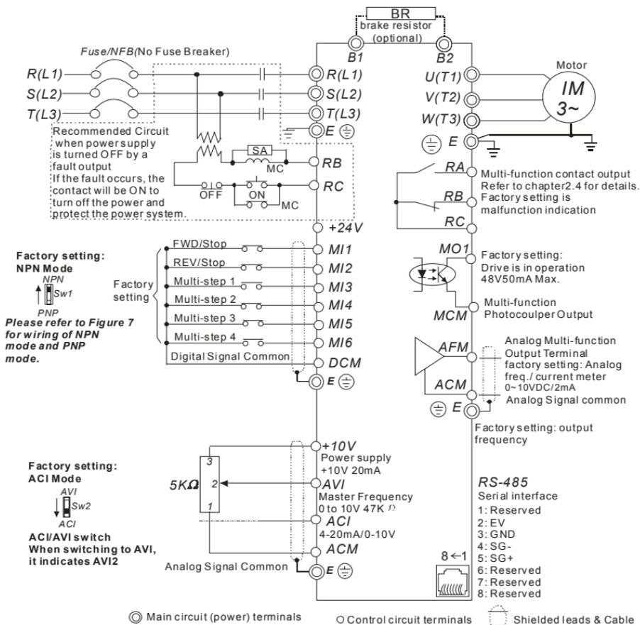
**NOTE** For VFD-E-T series, the braking resistor can be used by connecting terminals (B1 and B2) directly. But it can't connect DC-BUS in parallel.
