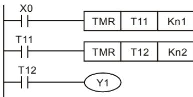
In this circuit, the total delay time from input X0 is close and output Y1 is ON=  $(n1+n2) \times T$ , where T is clock period.
