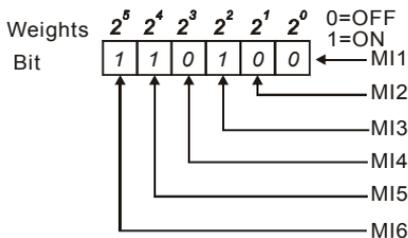
When extension card is installed, the number of the digital input terminals will increase according to the extension card. The maximum number of the digital input terminals is shown as follows.
