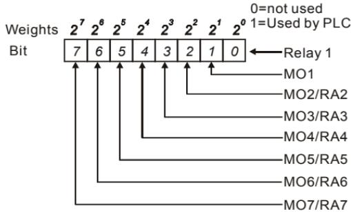
For example: when Pr.03.09 is set to 3 (decimal) = 00000011 (binary) that indicates Relay 1 and MO1 are used by PLC. (Pr.03.09 =  $2^0 + 2^1 = 3$ )
