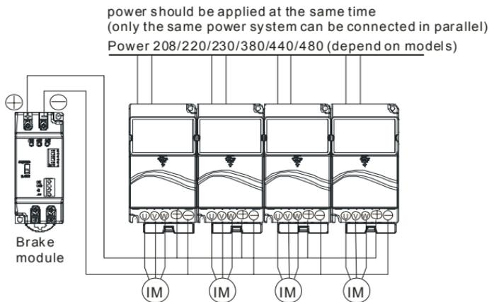
For frame A, terminal + (-) is connected to the terminal + (-) of the brake module.
