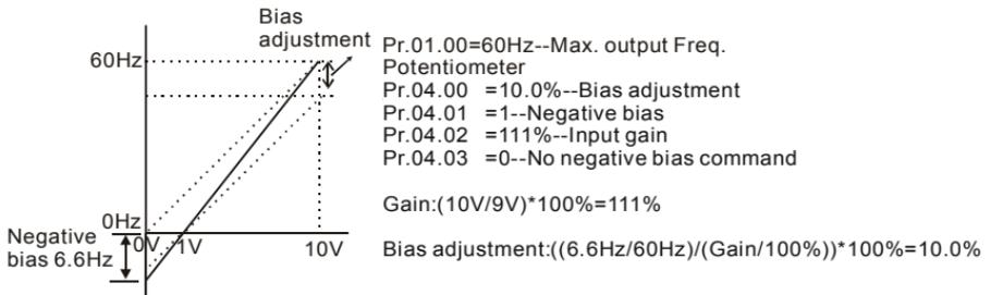
**Example 7: Use of 0-10V potentiometer signal to run motor in FWD and REV direction**
