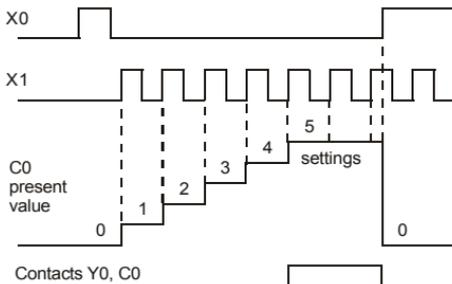
32-bit high-speed addition/subtraction counter C235:
