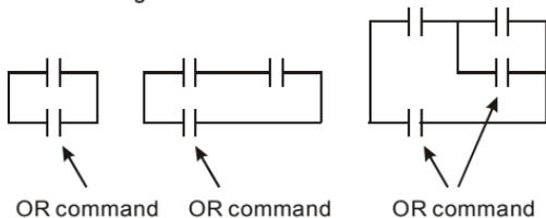
The structures of ORP and ORF are the same but the action is in rising-edge or falling-edge.
