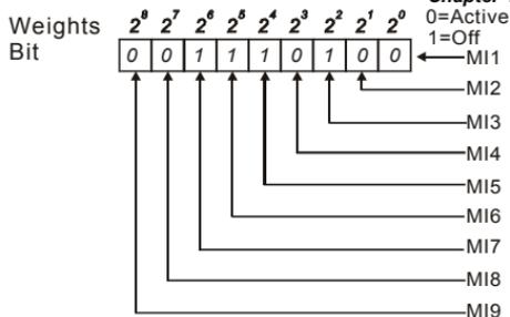
When extension card is installed, the number of the multi-function input terminals will increase according to the extension card. The maximum number of the multi-function input terminals is shown as follows.
