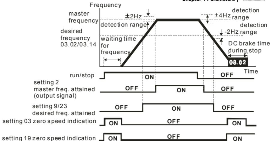
output timing chart of multiple function terminals
