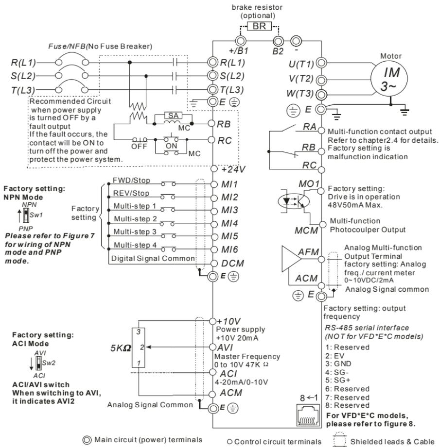
Figure 5 for models of VFD-E Series
