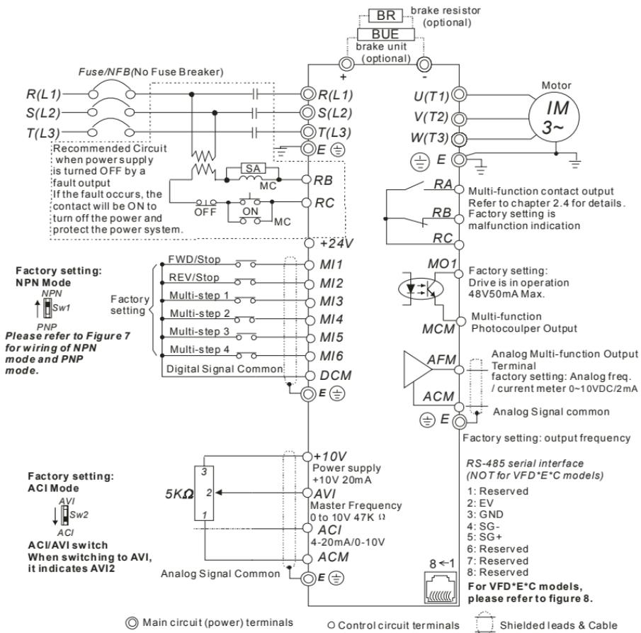
Figure 3 for models of VFD-E Series
