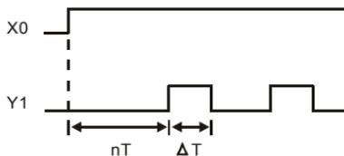
The figure above uses timer T0 to control coil Y1 to be ON. After Y1 is ON, timer T0 will be closed at the next scan period and output Y1. The oscillating circuit will be shown as above. (n is the setting of timer and it is decimal number. T is the base of timer. (clock period))
